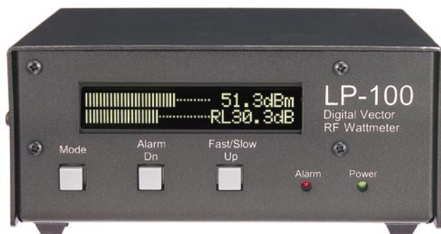
Figure 5 — The LP-100's front panel readout can display power in dBm and return loss in dB in addition to power in watts and SWR. In the vector mode, the display shows impedance. The top line is magnitude and phase, and the bottom line shows resistive and reactive components.
