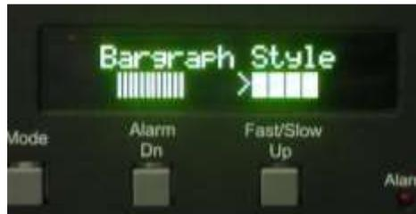
This is done by pressing the third button on the LP-100. If you have very old firmware, you may not have this option, in which case you must flash new firmware to see anything on your new display. After making the selection, you must power the meter down and back up.
